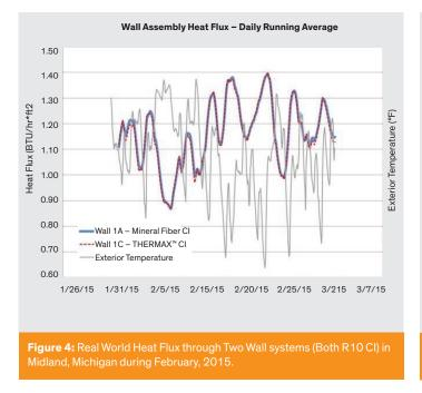
There are three lines on this graph of the thermal performance of these wall systems, but it is hard to tell since it looks like there are only two. The gray line indicated the exterior air temperature measured every hour during the month. We would expect to see the amount of heat driven through the wall to increase when the outside air temperature decreases due to the greater temperature difference across the wall assembly, and that is exactly what we see.
