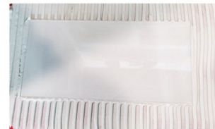
Transparent plexiglass simulates a tile laid in thin set mortar applied with a one direction motion of the notched trowel. Note the deep embedment of the tile due to the ease of mortar ridge collapse.
